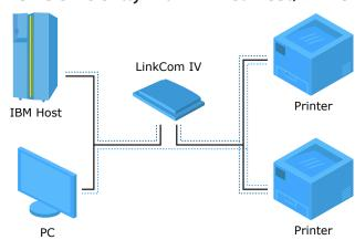
LinkCom IV is developed to work efficiently within the mixed Host/LAN environment and supports SNA and TCP/IP sessions directly from the IBM systems as well as TCP/IP sessions from the LAN. The LinkCom IV will convert IBM SCS/DCA and IPDS to the industry standard
